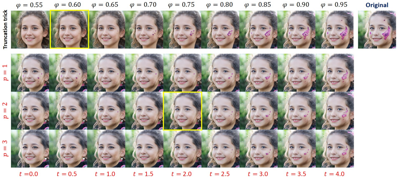
Figure 8. Choice of hyper-parameters. Top row: images generated with truncation trick with \psi = 0.55 to 0.95 . Rows 2-4: images generated with our method with t = 0.0 to 4.0 , p = 1 to 3 . Our method removes the artifacts while retaining almost all important features of the original image, indicating that it achieves a better trade-off between image quality and diversity than the truncation trick.
