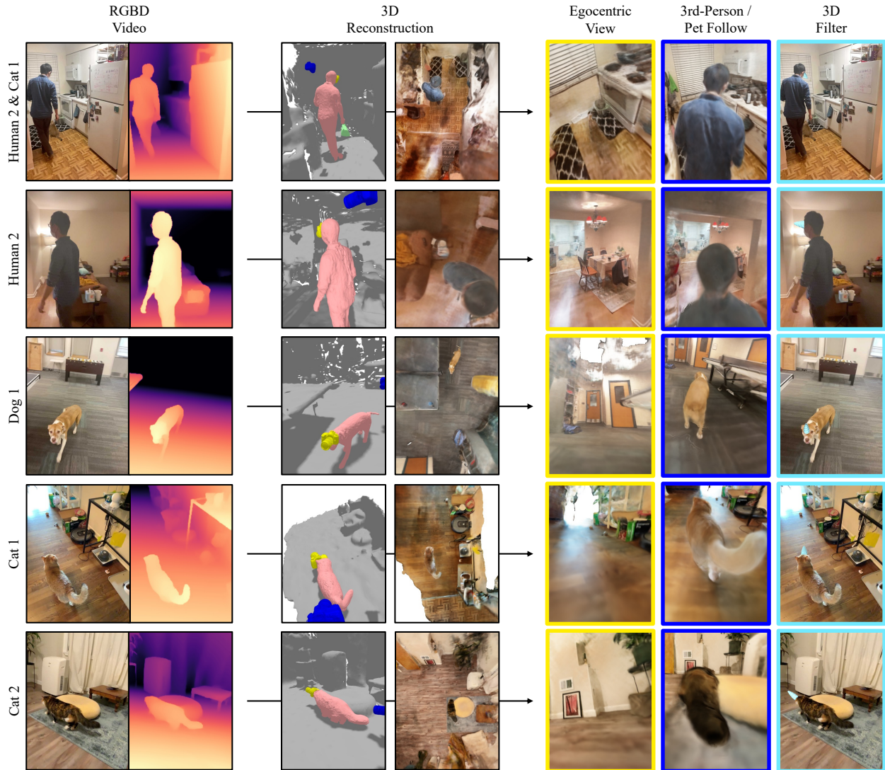
Figure 4: Embodied View Synthesis and 3D Filters. For select sequences of our RGBD dataset, we visualize the scene geometry and appearance reconstructed by our method (3D reconstruction) and the resulting downstream applications. The yellow and blue camera meshes in the mesh renderings represent the egocentric and 3rd-person-follow cameras, respectively. To showcase the 3D video filter we attach a sky-blue unicorn horn to the forehead of the target object, which is then automatically propagated across all frames. Full-length videos can be found at https://andrewsonga.github.io/totalrecon/applications.html .
