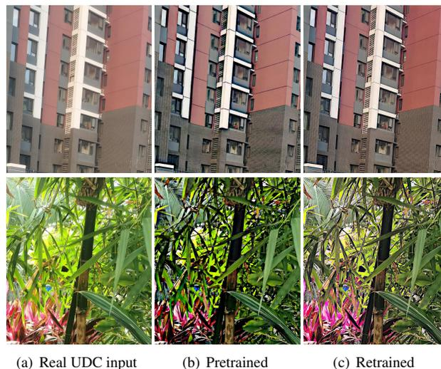
Figure 9. Comparison of BNUDC pretrained and retrained with synthetic data from different IFPs. (a) Real-world input UDC images. (b) Results of BNUDC pretrained with data generated by Feng *et al.* [6]. (c) Results of BNUDC retrained with data from our enhanced IFP. Our synthetic data effectively improves the visual quality of the restored results from BNUDC.
