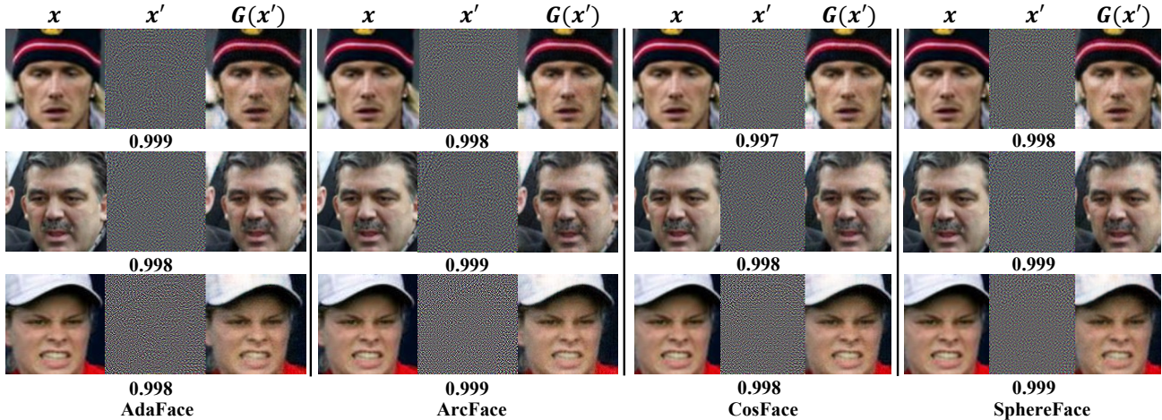
Figure 3. Adversarial Visual Information Hiding (AVIH) method protect face images for different service models. We mark below each protected image the cosine similarity between its feature vector and the original image’s feature vector.
