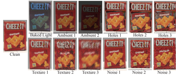
Figure 4: Example of cheezit object with each type of artifact applied from the YCB-Synthetic artifact datasets.
