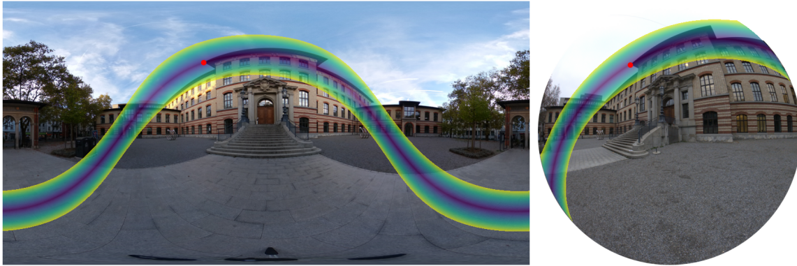
Figure 1. The figure shows the level sets of the proposed Tangent Sampson error. In contrast to classical Sampson error, the proposed error function applies to arbitrary central camera models; in this case a 360 panoramic image and a fisheye camera. Given a relative pose and a pair of points (highlighted in red), we vary a point on one image while keeping the other fixed, and thus get the values on each image. A given color corresponds to a constant value of reprojection error, with purple indicating near-zero errors along the epipolar curve.
