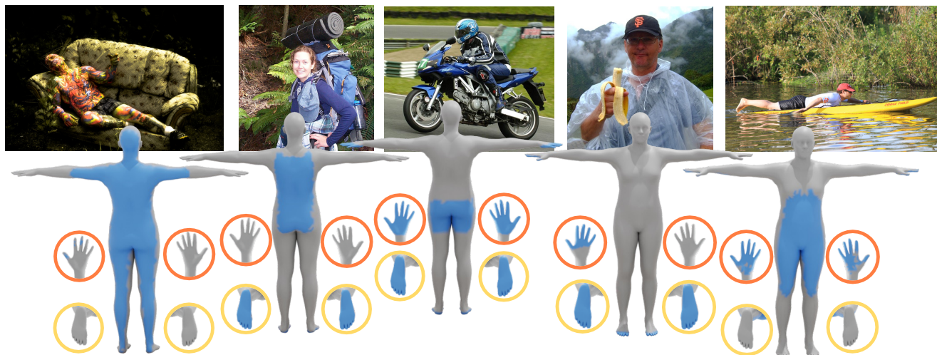
Figure 1: Given an RGB image, DECO infers dense vertex-level 3D contacts on the full human body. To this end, it reasons about the contacting body parts, human-object proximity, and the surrounding scene context to infer 3D contact for diverse human-object and human-scene interactions. Blue areas show the inferred contact on the body, hands, and feet for each image.
