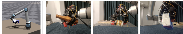
Figure 6: Real-world experiments with Allegro Hand Left: grasping in the simulator, Right: grasping in the real world.
