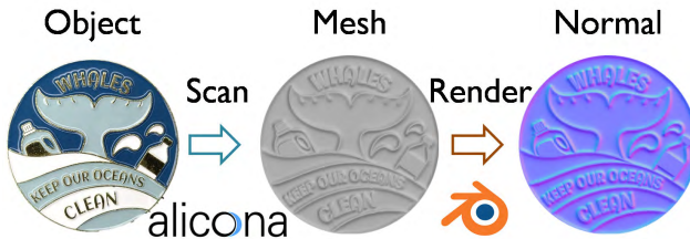
Figure 3: Process of obtaining a ‘GT’ normal map.
