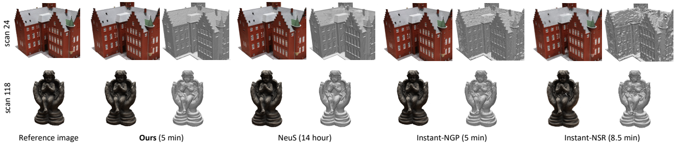
Figure 4. Qualitative comparisons on DTU dataset for static scene geometry reconstruction and novel view synthesis. Our method demonstrates high-quality rendering quality, superior to NeuS and comparable to Instant-NGP in terms of complex texture reconstruction. In addition, it outperforms all baselines regarding to 3D geometry reconstruction, with fine details without inducing noise.
