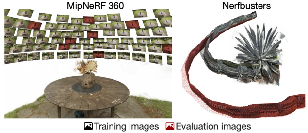
Figure 2: Evaluation protocols. Current evaluation of NeRFs (e.g., MipNeRF 360) measures render quality at every 8th frame of the captured (training) trajectory, thus only testing the model’s ability to render views with small viewpoint changes. In contrast, we propose a new evaluation protocol, where two sequences are captured of the same scene: one for training and one for evaluation. Please see the supplementary material for plots showing the training and evaluation sequences for various NeRF datasets, including our proposed Nerfbuster Dataset.
