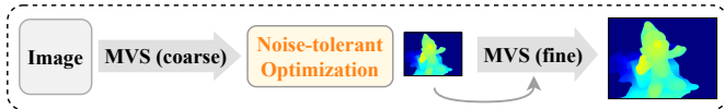
Figure 2. Our proposed method improves the quality of depth maps obtained from the coarse stage multi-view stereo (MVS) by introducing noise-tolerant optimization techniques. The resulting depth maps then guide depth hypothesis sampling in the finer stage MVS, leading to more accurate and detailed 3D reconstructions.
