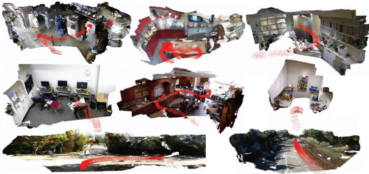
Figure 1: Robust 3D scene reconstruction of challenging and diverse scenes. Given a monocular video, our algorithm reconstructs the 3D scene without requiring offline-acquired camera poses. Significantly, our approach only involves dozens of parameters of each frame to optimize online. Here, the red triangulations denote the estimated camera trajectories.
