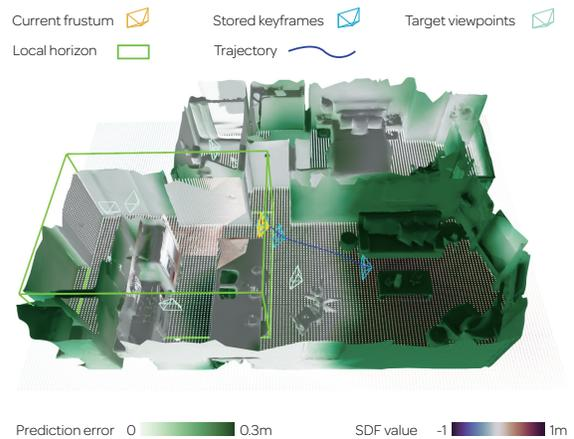
Figure 1: An overview of the proposed active neural mapping system. Guided by the continually-updated neural map (visualized as the SDF values through a forward pass), the mobile agent explores the environment actively to minimize the prediction uncertainty (visualized as the prediction error given the truth surface points).
