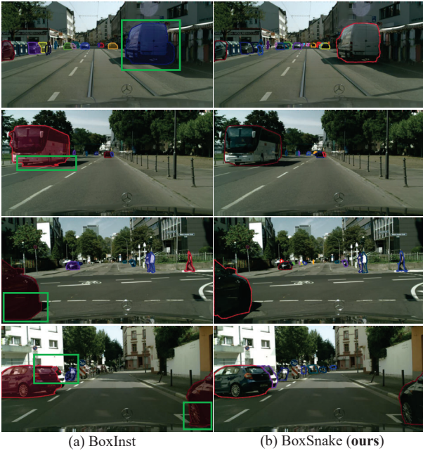
Figure 6. Qualitative comparisons on Cityscapes validation set. The major difference is marked by the green rectangle.
