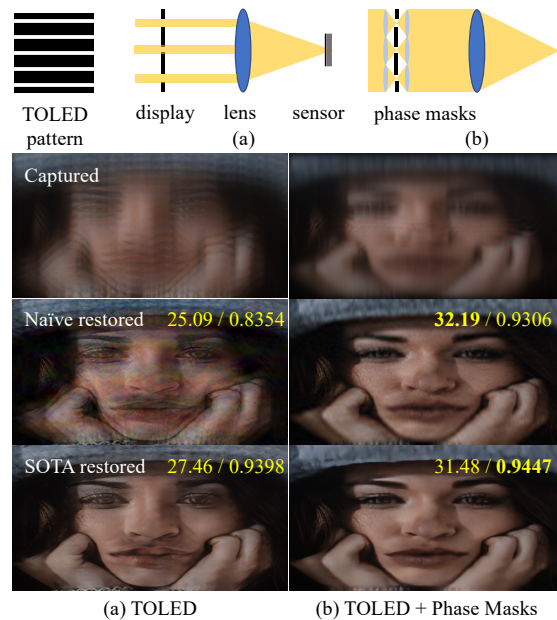
Figure 1: A comparison between a UDC under a transparent-OLED display (a) without and (b) with the proposed phase masks. (From top to bottom) Rows show the setup, images captured under each, restored images using a naive iterative solver, and using a state-of-the-art deep network [5]. We show PSNR(↑) in dB and SSIM(↑) for restored images. Both UDCs have a pixel density of 600 DPI.
