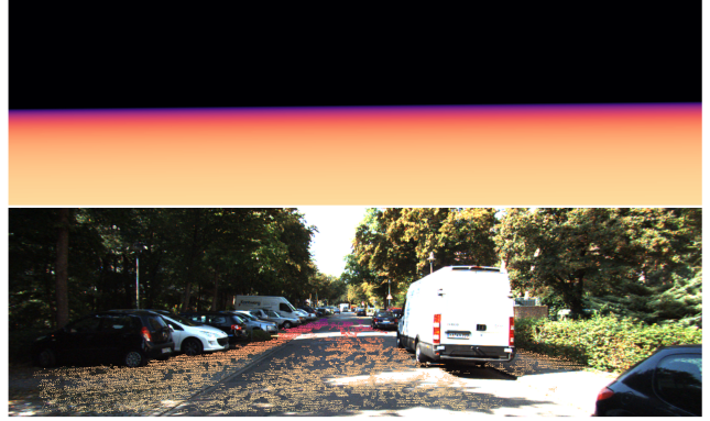
Figure 4. Top demonstrates the ground depth calculated from camera parameters (the dark region above the vanishing line indicates infinite depth). Bottom visualizes the pixels of which ground depth values are sufficiently close (i.e., relative error < 3\% ) to the sparse ground-truth values provided by LiDAR in KITTI.
