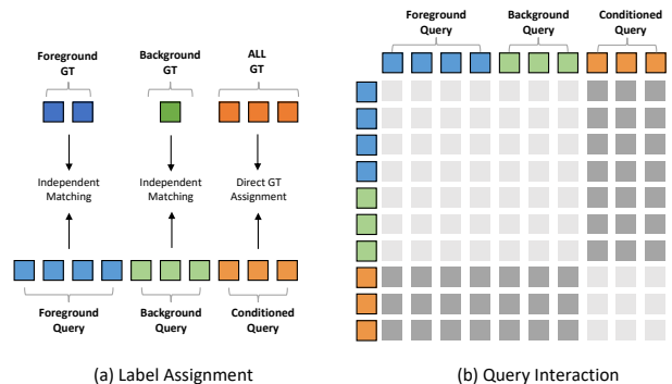
Figure 4: a) Label assignment for different queries. “gray” means unused for detection data without background stuff. Best viewed in color. b) Query interaction of different queries (foreground, background, and conditioned query) in OpenSeeD . All data has background queries including detection data. “dark” color means blocking interaction.
