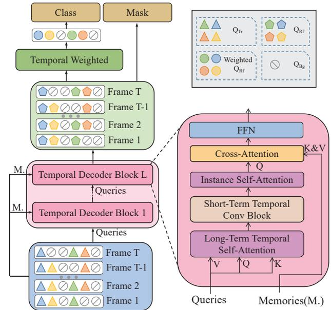
Figure 3. **The framework of the temporal refiner.** Instance representations for each frame ( $Q_{Rf}$ ) are denoted by pentagons, while the instance representations for the entire video ( $\hat{Q}_{Rf}$ ) are denoted by circles. Different colors indicate different instance IDs.
