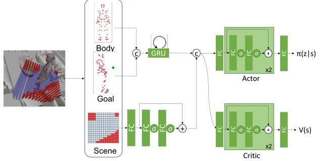
Figure 3: Illustration of the scene-aware locomotion policy network. The locomotion policy state consists of the body vectors from the markers, the goal-reaching feature of normalized direction vectors from markers to the goal pelvis, and the interaction feature of a 2D binary map indicating the walkability (red: non-walkable area, blue: walkable area) of the local  $1.6m \times 1.6m$  square area. The locomotion policy network employs the actor-critic architecture and shares the state encoder.
