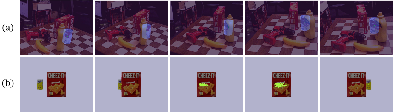
Figure 5. 3DNEL’s probabilistic formulation enables robust object pose tracking under occlusion with particle filtering. Green dots visualize the particles used to estimate posterior distributions in particle filtering. (a) 3DNEL can track objects through heavy occlusions. (b) 3DNEL can accurately quantify uncertainty (shown by the spread-out particles), which enables tracking through extended occlusions.
