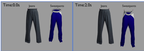
Figure 4. A visualization of different trousers with two grasping points on the waistband under gravity.
