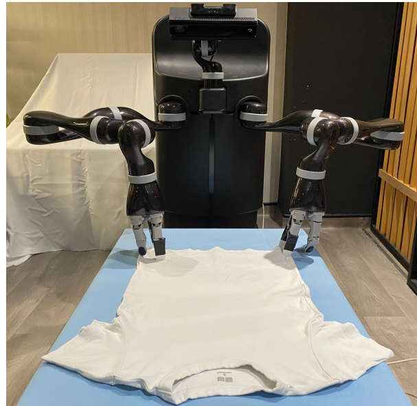
Figure 9. A visualization of our real-world experiment. We collect the point cloud from the RGB-D camera integrated within the MOVO as its head and control the two arms of MOVO to fold the t-shirt.
