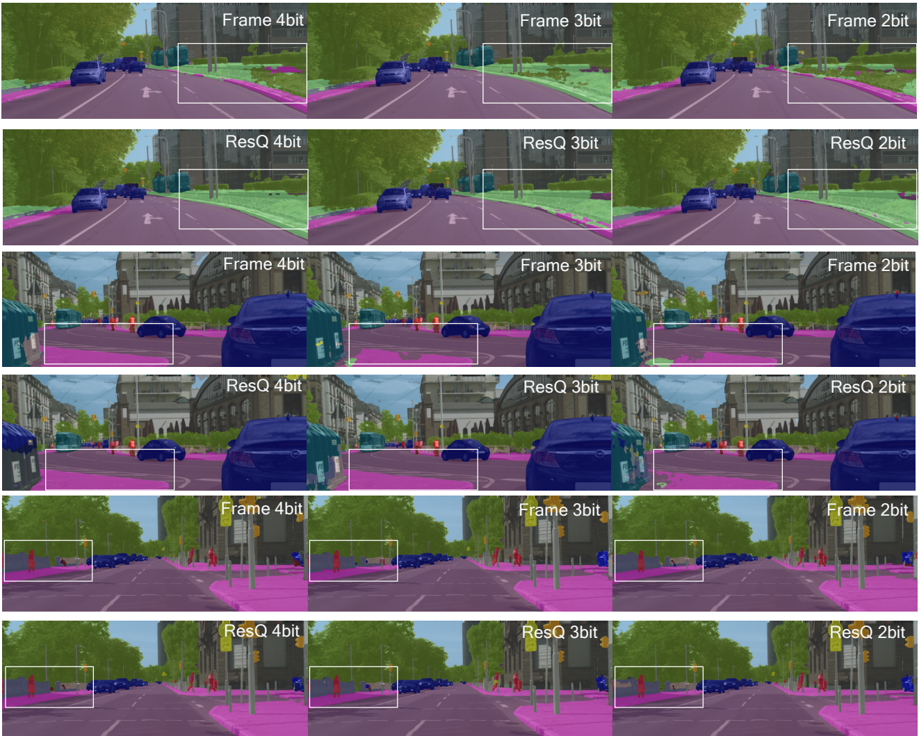
Figure 4. Qualitative comparison between frame and residual quantization at low bit-width. All models illustrated here benefit of QAT. In highlighted regions, our proposal significantly outperforms the baseline.
