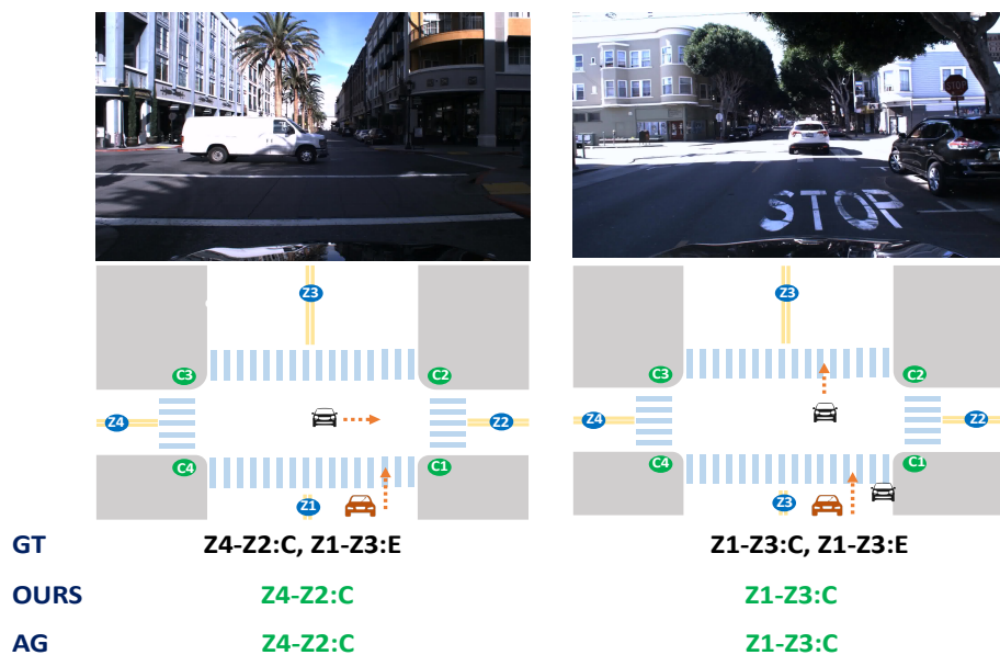
Figure 4: Qualitative results for multilabel atomic activity recognition of our method against ARG [4]. All ground truths contain ego vehicle action, i.e. activities starting with 'E' just for reference and it is not used for classification. The GT denotes ground truth, and green and red color denote true and false positives respectively.
