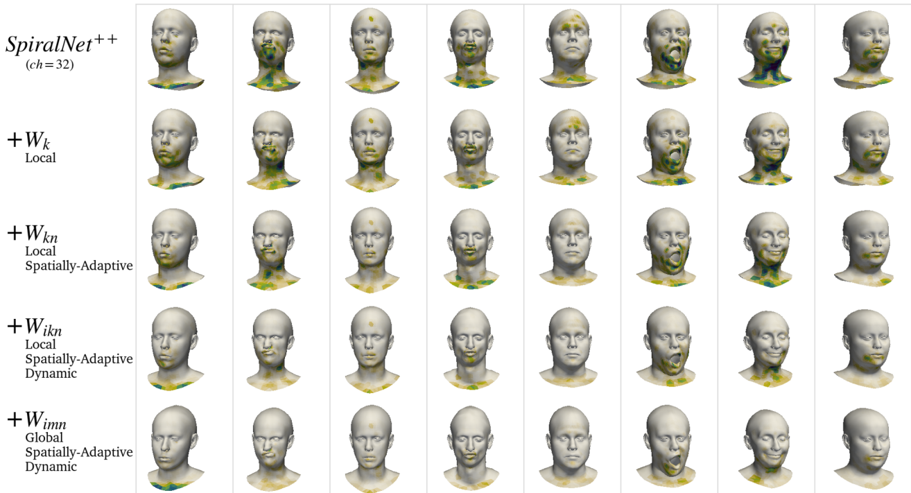
Figure 6: Qualitative comparison of 3DMM with different inductive biases. Visualization of the per-vertex euclidean distance from ground truth (mm) for a SpiralNet^{++} baseline ( ch=32 ) augmented with different layers. Errors are saturated at 10mm. Each layer incorporates a different characteristic in the model. Observing each example from the top row to the last row highlights the contribution of each new characteristic to the 3DMM. The last row shows how the integration of non-local reasoning, vertex-wise adaptivity ( i.e. spatially-adaptive), and instance-wise adaptivity ( i.e. dynamic) achieves the lowest reconstruction error.
