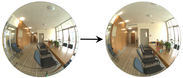
Figure 1. To compute the illuminance of the image, the geometric calibration of the camera is used to project the captured HDR (left) to an orthographic projection (right).
