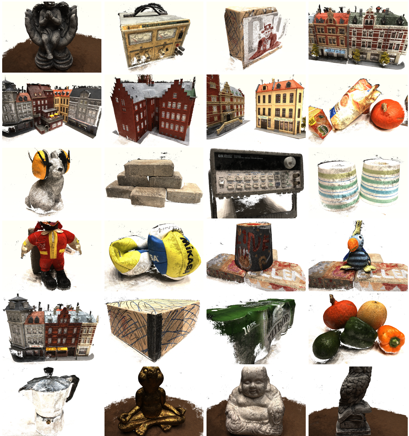
Figure S.9. Output point clouds of V-FUSE from the DTU [1] dataset using NP-CVP-MVSNet [8] as input.
