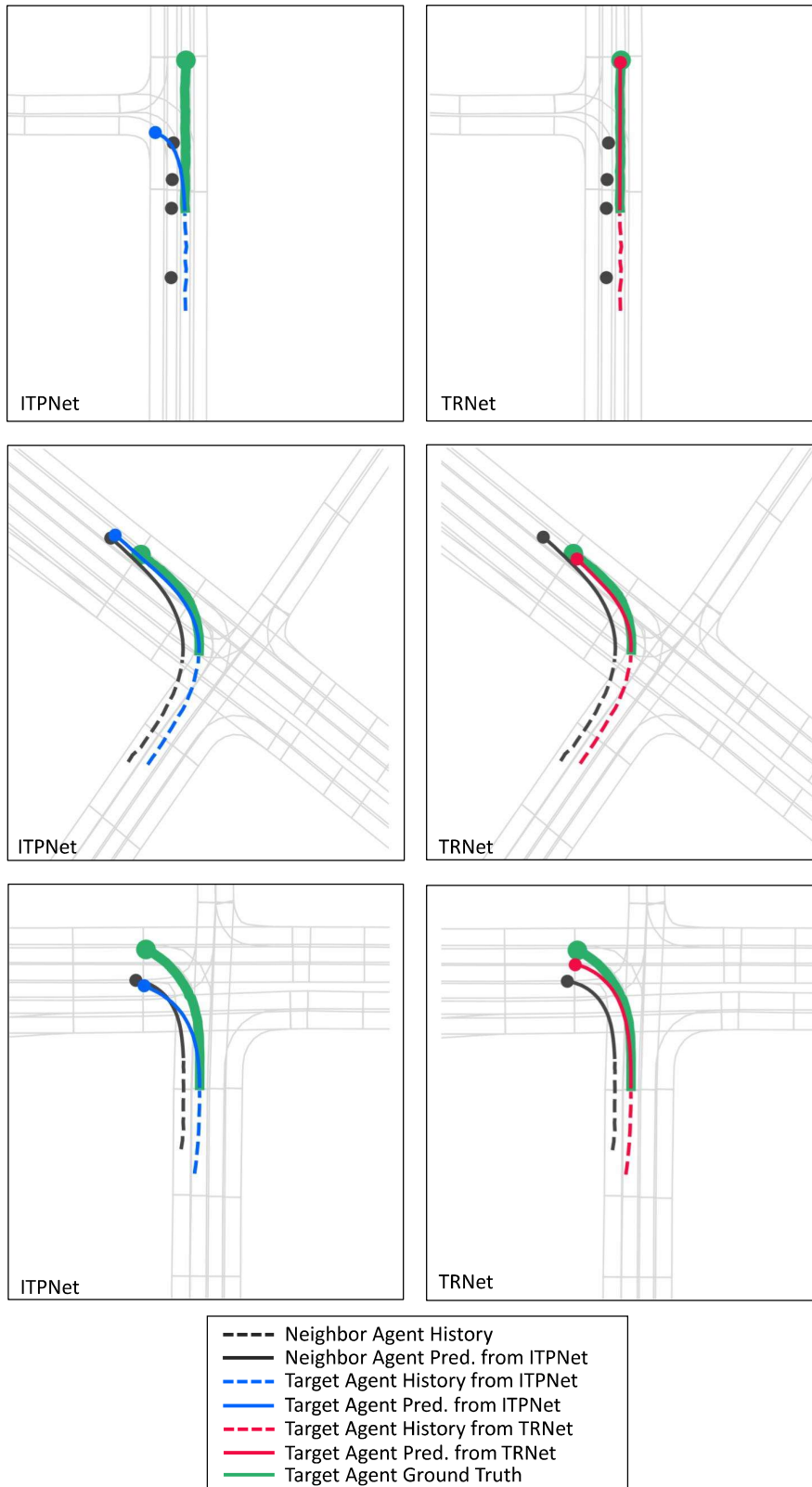
Figure 5. Visualization of trajectories for several intersection scenarios. The target agents interact with the other agents at intersections. For all cases considered, TRNet produces trajectories that do not collide with other trajectories.
