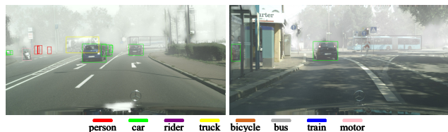
Figure 5. Illustration of some failure examples. The bus with large aspect ratios cannot be detected well.
