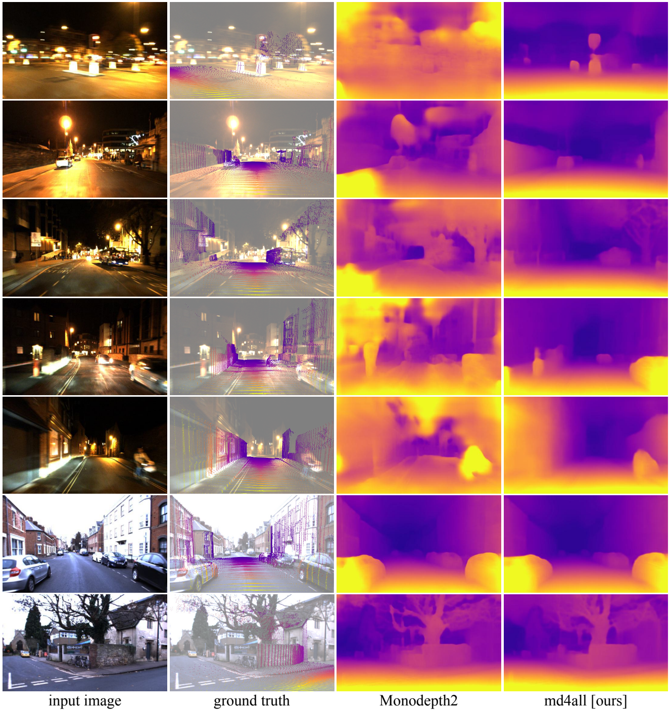
Figure 15. Comparison of self-supervised models on RobotCar [10] night and day samples. The standard Monodepth2 [7] is compared to our md4all-DD applied to Monodepth2.
