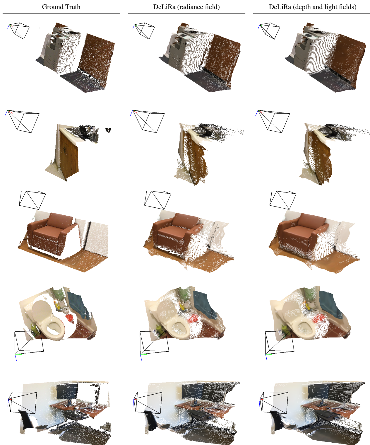
Figure 5: Qualitative depth and view synthesis results from unseen viewpoints, using different DeLiRa decoders. The first column shows ground truth point clouds, while the second and third columns show respectively pointclouds generated using radiance field predictions, and depth and light field predictions.
