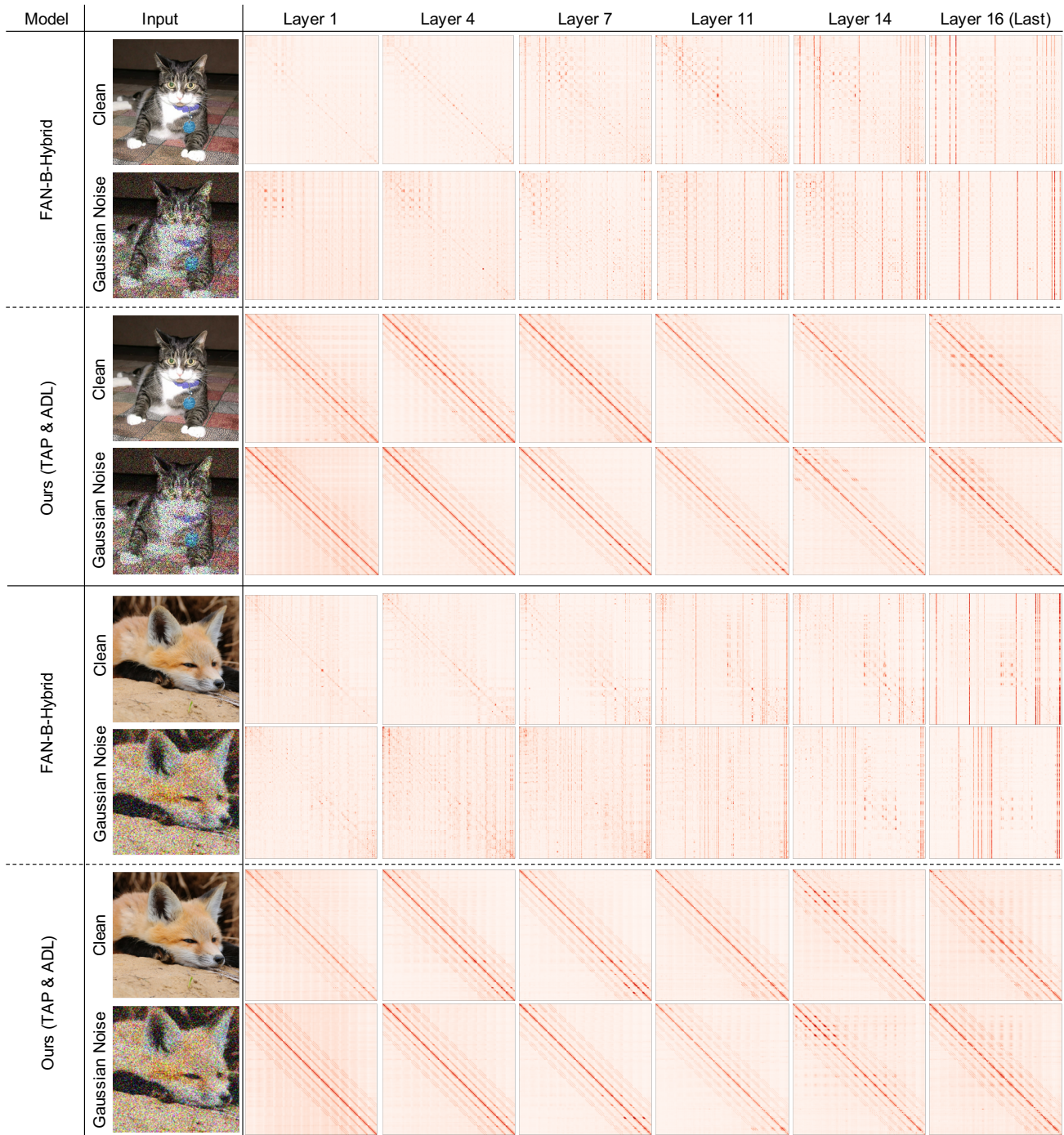
Figure I. Attention maps of intermediate layers based on FAN-B-Hybrid. We demonstrate that the token overfocusing issue can be observed in most layers and becomes gradually more serious with the increase of depth. When facing common corruptions, e.g., Gaussian noise, the attention mechanism becomes extremely fragile by focusing on entirely different important tokens. By contrast, our model follows a similar attention pattern (diagonal) across layers and exhibits better stability against corruptions.
