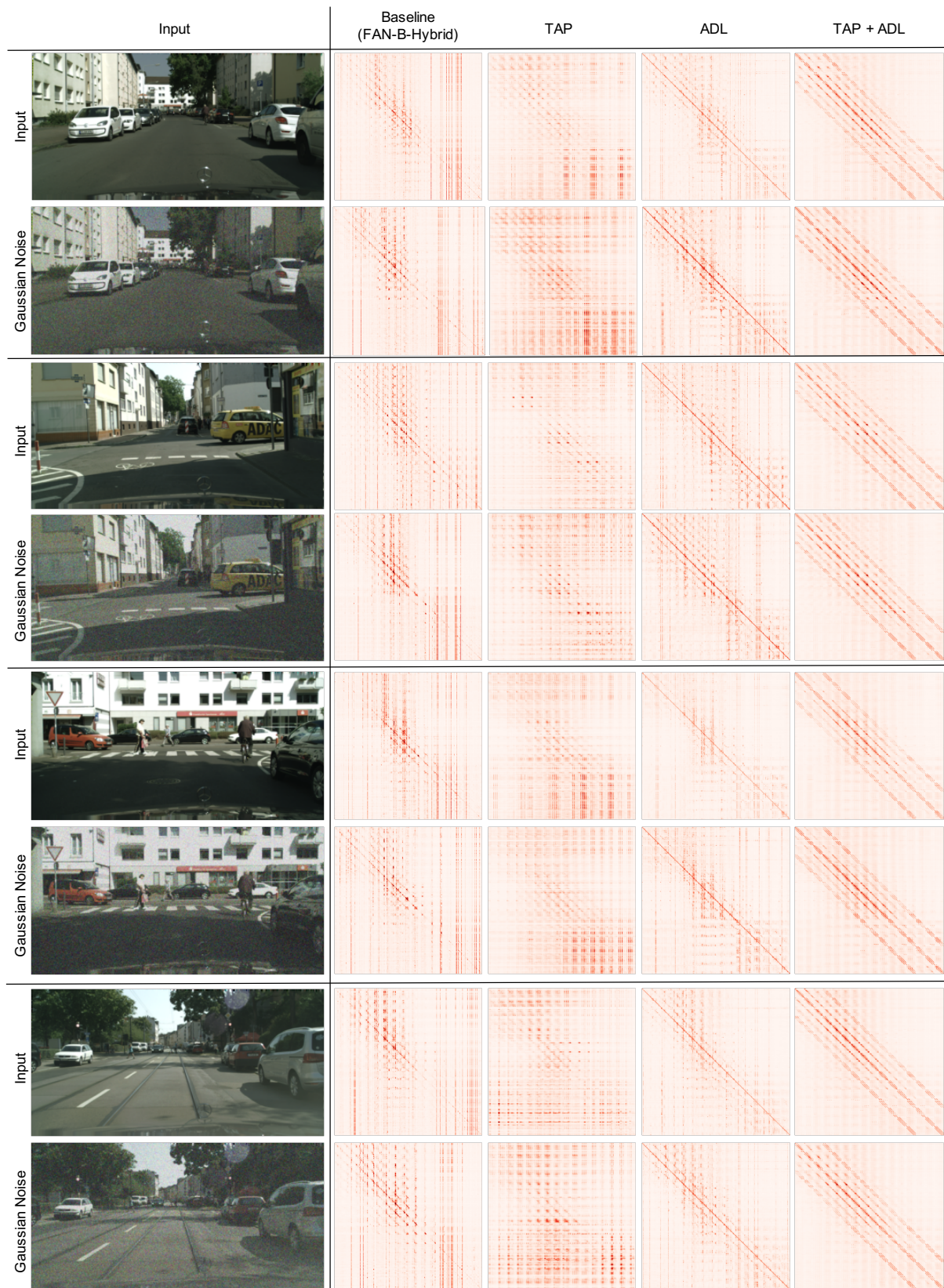
Figure IV. Attention maps of the last layer in the segmentation model based on FAN-B-Hybrid backbone. We show that the token overfocusing issue also exists in segmentation models and the attention mechanism is very fragile to image corruptions. By contrast, our TAP and ADL obtains consistent attention pattern for both image classification and semantic segmentation models. These results indicate the generalization ability of our approaches to the semantic segmentation tasks.
