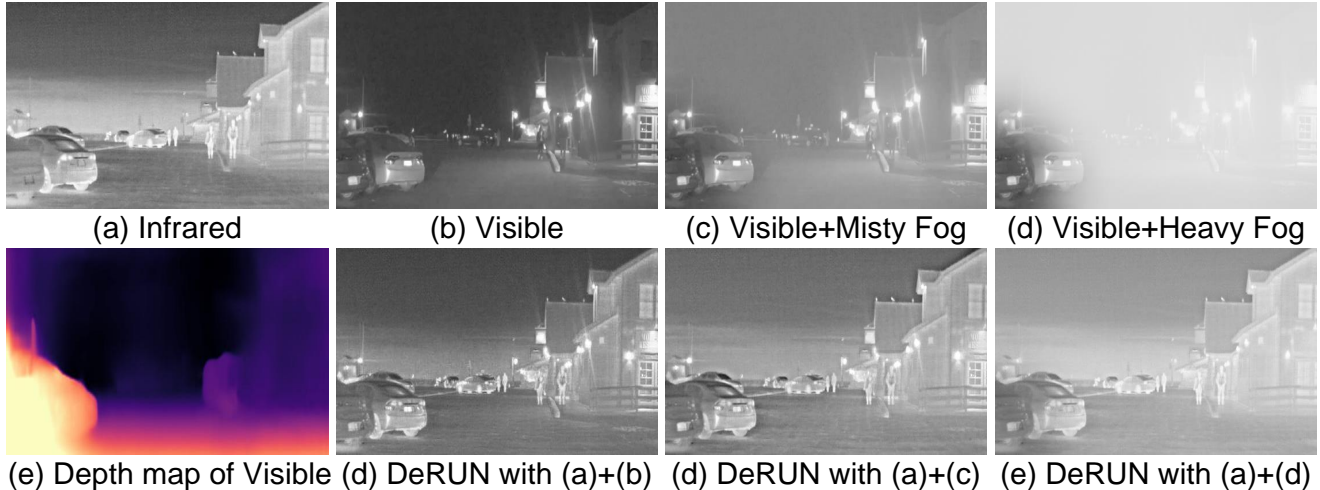
Figure 2: Failure cases of DeRUN. We simulate misty fog and heavy fog on the visible image (b) based on its depth map (a), where DeRUN fails to enhance part of the salient texture information under the scenario with heavy fog.
