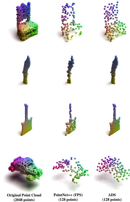
Figure 8. Qualitative comparison on ShapeNetPart. The visual results demonstrate the proposed method and basic PointNet++ on a dense Part segmentation example.
