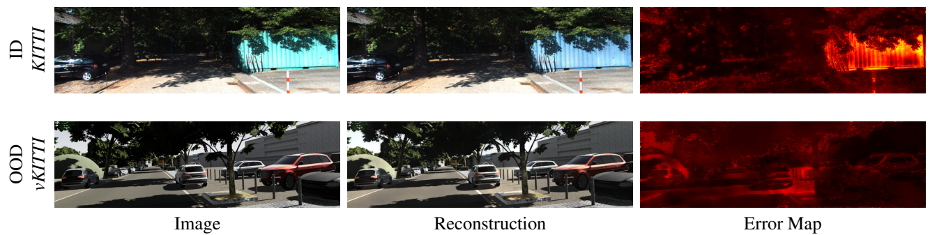
Figure 6: Failure of the image decoder for in-distribution (ID) image from KITTI [4] and out-of-distribution (OOD) image from virtual KITTI (vKITTI) [2] as input to Monodepth2 [5] trained on KITTI [4].
