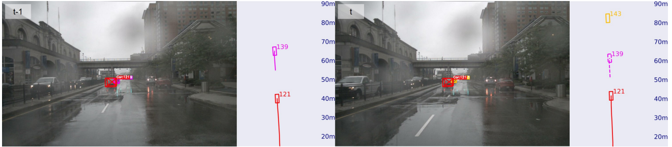
Figure 2. Representative failure case. The solid lines and boxes denote the tracking results for timestamps t - 1 and t , while the dotted one is the mismatched tracklet (#139) in the coordinate at t timestamp. The failure case is caused by the inaccurate observation (yellow box at frame t ) from the monocular 3D object detector. The tracker cannot associate the detection with any tracklet (e.g., #139), thus generating a new identity for it (#143). Note that, we only plot a few bounding boxes for better illustrations in this example.
