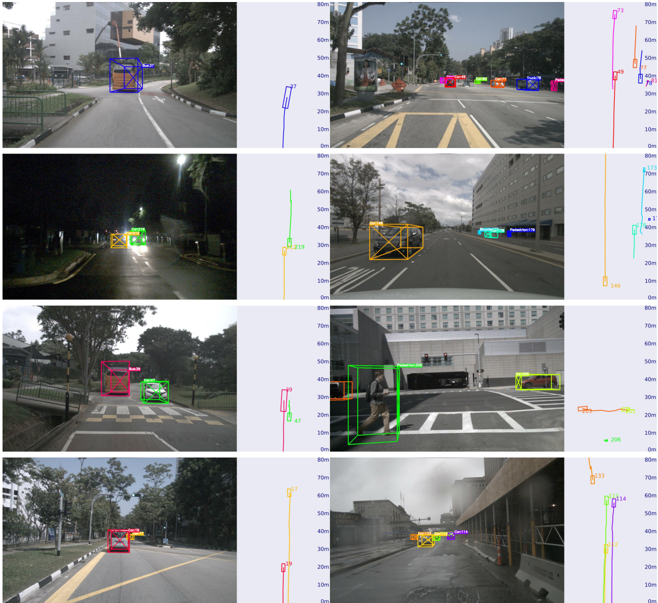
Figure 1. Qualitative results on the nuScenes validation set. We plot the tracking results of our MoMA-M3T based on the image view (left) and the bird’s eye view (right) with the 15 historical frames on the BEV plane, in which different colors denote different tracklets.
