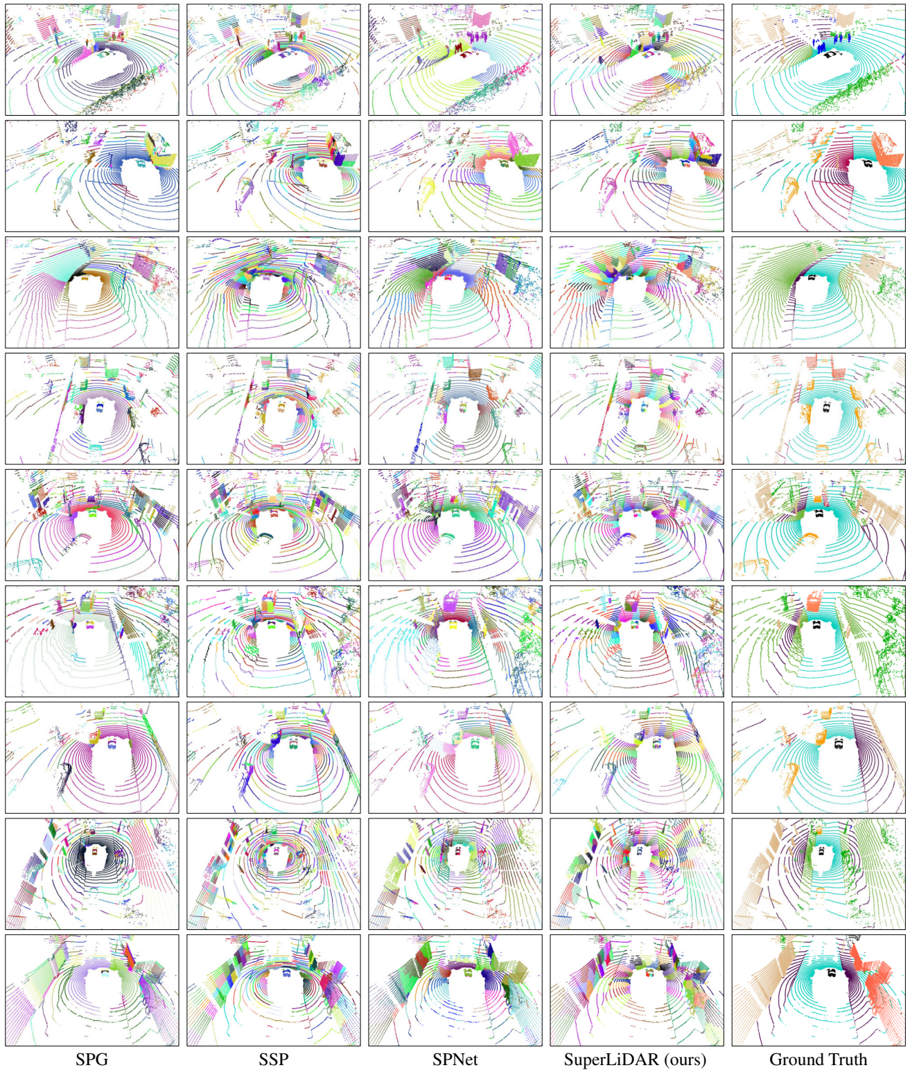
Figure 4. Visualization of superpoints generated by different methods on the validation set of nuScenes. Note that the superpoints are randomly colored (zoom in for a better view).
