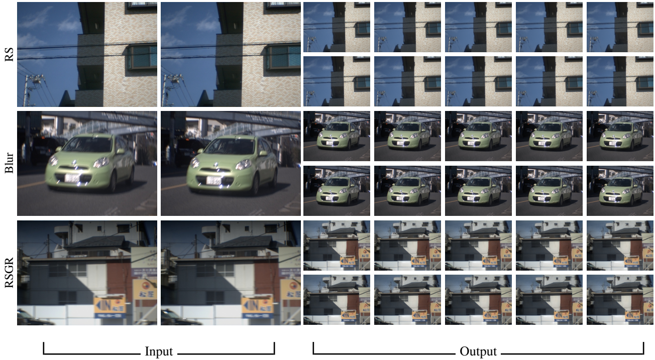
Extended Figure B.6: Reconstructed consecutive frames from two degraded inputs by using DeMFI. We present the multiple intermediate frames at different time generated by three types of shutter induced degradations. They are temporally located at t = [0, 1) with stride of 0.1 and arranged in two rows from left to right. Best viewed in zoom.
