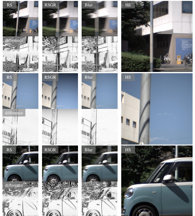
Extended Figure A.2: Data samples of different degradations under the same scene from our RD-VFI. On the left, original images are on the top row and corresponding difference maps computed with the HS frame are at bottom.
