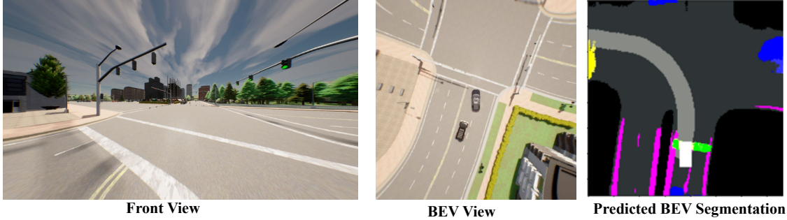
Figure 1: Visualization of the inertia issue where the behavior cloning-based agents often fail. The agent fails to proceed despite the green traffic light, blocking the other car behind.
