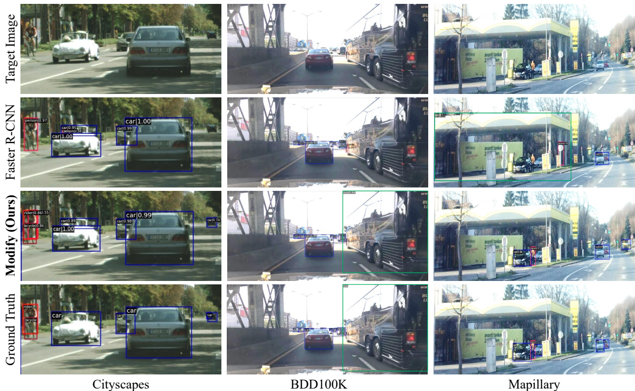
Figure 2: Qualitative results of the object detection task for the setting of training on SYNTHIA and validating on Cityscapes (Column 1), BDD100K (Column 2), and Mapillary (Column 3), respectively. Zoom in for a better view.
