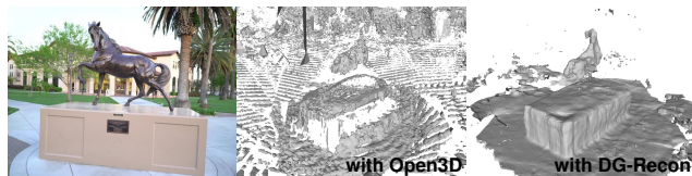
Figure 6. Outdoor reconstruction example: Horse [12]. Note that relative depths from Omnidata were scaled with COLMAP sparse depths to obtain metric depths.
