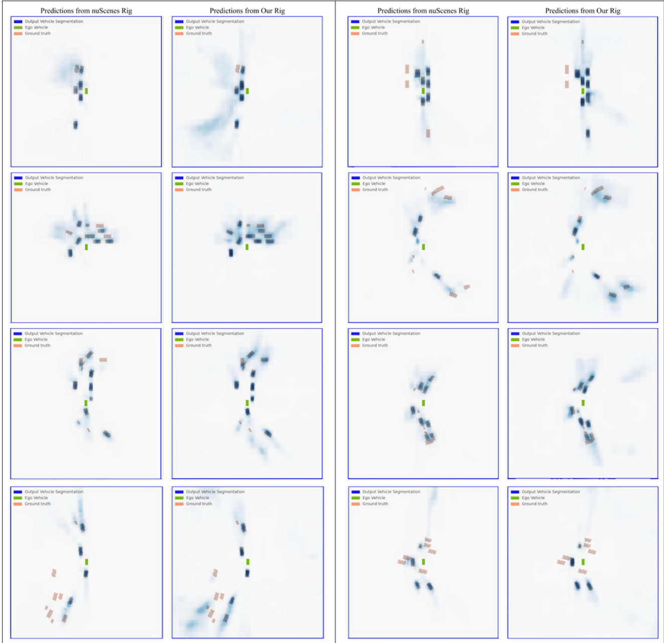
Figure 6: BEV Segmentation Predictions: Visualizations of the predictions made by a BEV segmentation model trained with data from the nuScenes rig (left) compared to our CD-optimized rig (right) on the same test scene. We observe that, on the same scenes, predictions from our rig are, in general, more accurate and have higher confidence.
