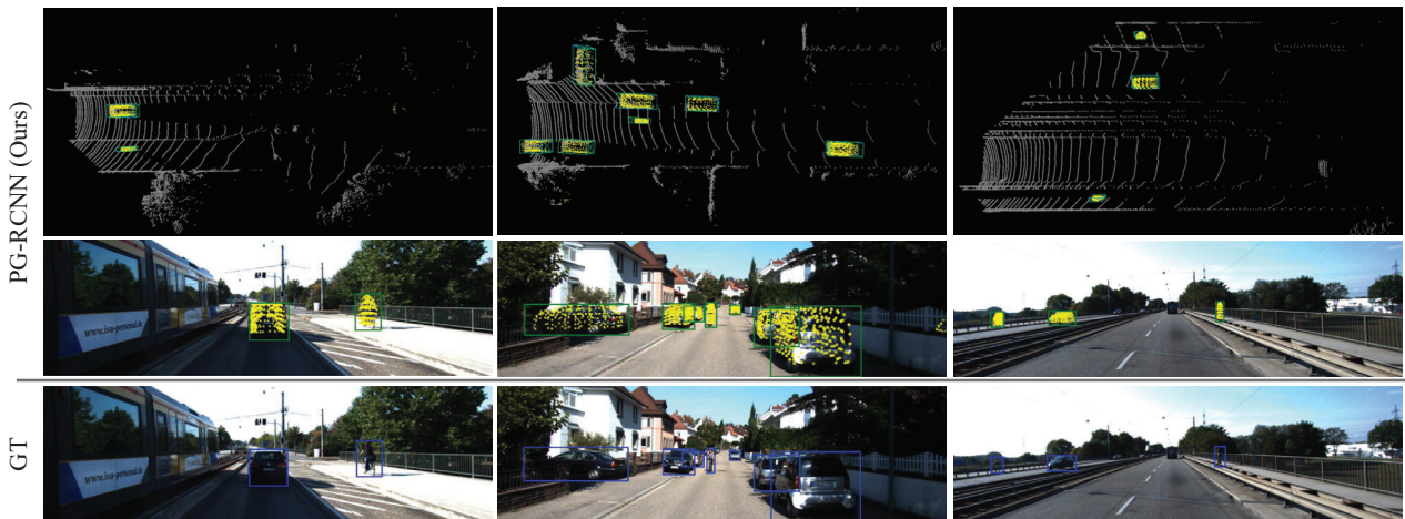
Figure S3. More qualitative results on KITTI dataset. The generated points, predicted bounding boxes, and ground truth bounding boxes are highlighted in yellow, green, and blue, respectively.
