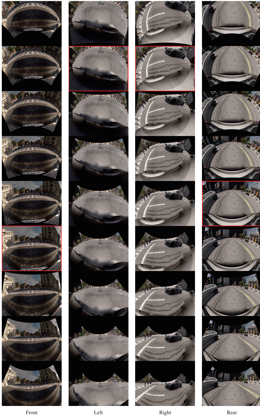
Figure 2: Examples of the augmented fisheye images on the SynWoodscape dataset. Black areas indicate the regions beyond the field of view of the original fisheye images. Red boxes in each column denote original images, and the other images are augmented images.
