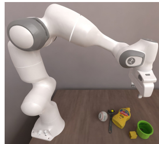
Figure 1: Illustration of the PickClutter task. Given the name of a target object, the robot agent needs to decide whether the corresponding object is graspable based on the current visual observation.
