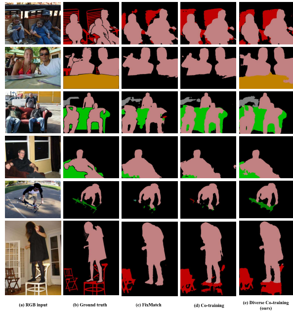
Figure 10. Example qualitative results from PASCAL VOC 2012 . (a) RGB input; (b) ground truth; (c) FixMatch; (d) Co-training baseline; (e) Diverse Co-training (ours). (c) and (d) use DeepLabv3+ with ResNet50 as the segmentation network while (e) uses DeepLabv3+ with ResNet50 and SegFormerb2 (with MLP head) as the two segmentation networks.
