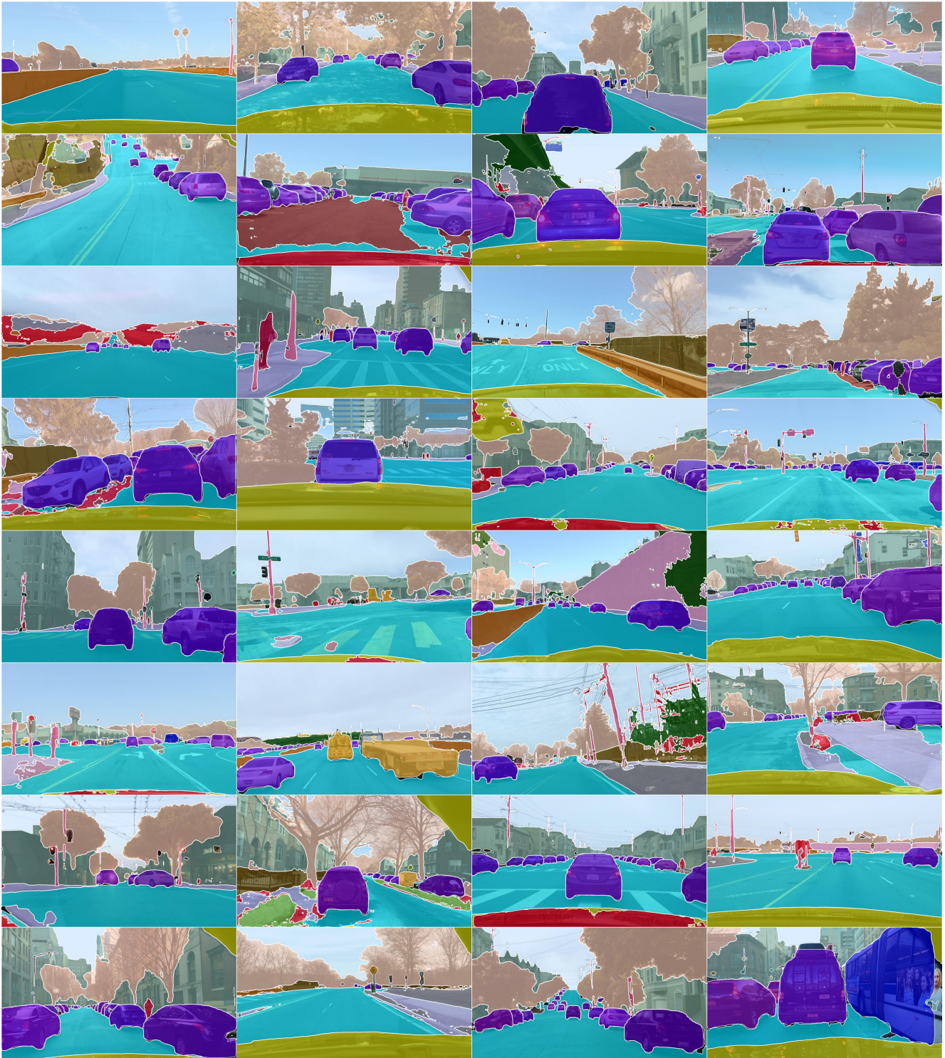
Figure 18. BDD100K panoptic segmentation visualization: pre-trained with DreamTeacher feature distillation on IN1k-1M. The backbone is resnet-50, finetuned using PanopticFPN. Only the backbone weight is pre-trained, other part of the networks are randomly initialized.
