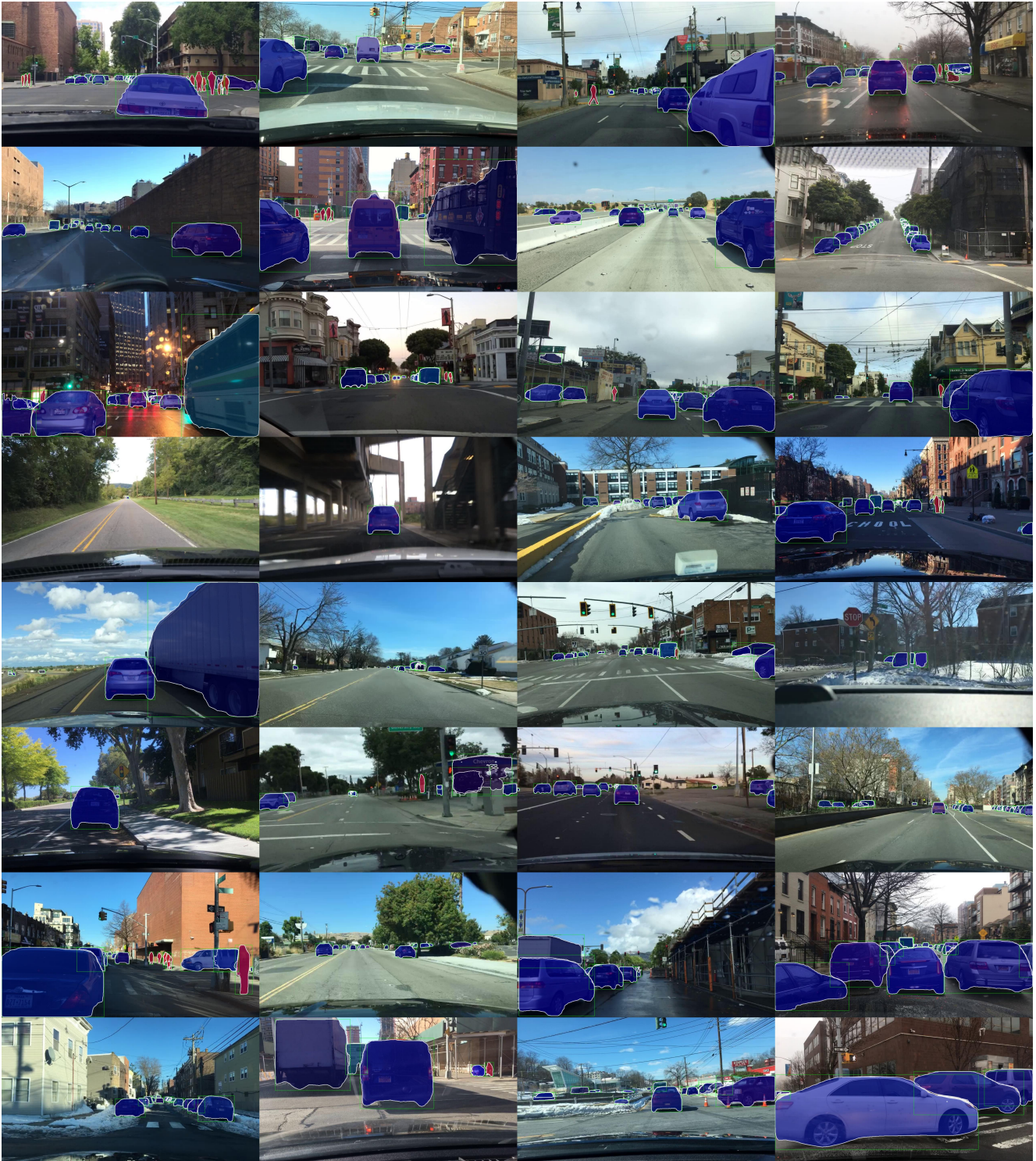
Figure 16. BDD100K instance segmentation visualization: pre-trained with DreamTeacher feature distillation on IN1k-1M. The backbone is resnet-50, finetuned using Mask R-CNN. Only the backbone weight is pre-trained, other part of the networks are randomly initialized.
