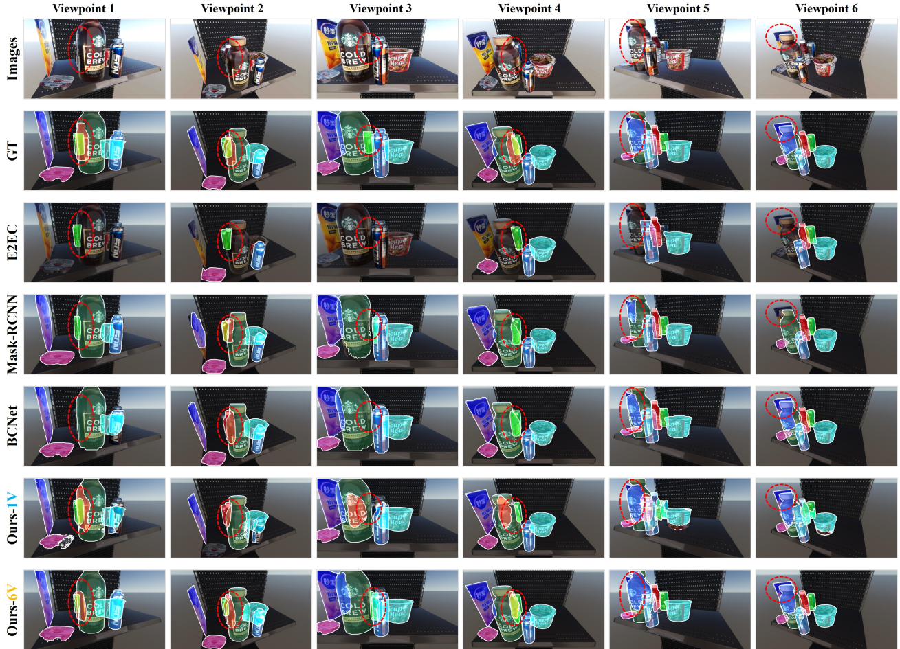
Figure 2: The second example of comparison between state-of-the-art methods and ours on MUVA, trained with one viewpoint (1V) and six viewpoints (6V). For masks, different colors denote different instances, and the same instance in different angles has the same color. Red circles indicate regions should be focused. Zoom in for a better view.
