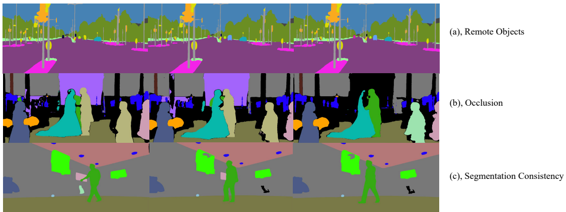
Figure 4: Visual Results on Failure Cases of Tube-Link. (a), Remote objects lead to ID switches and inferior segmentation results. (b), Heavy occlusion leads to an ID switch. (c), Segmentation consistency problems caused by camera motion.
