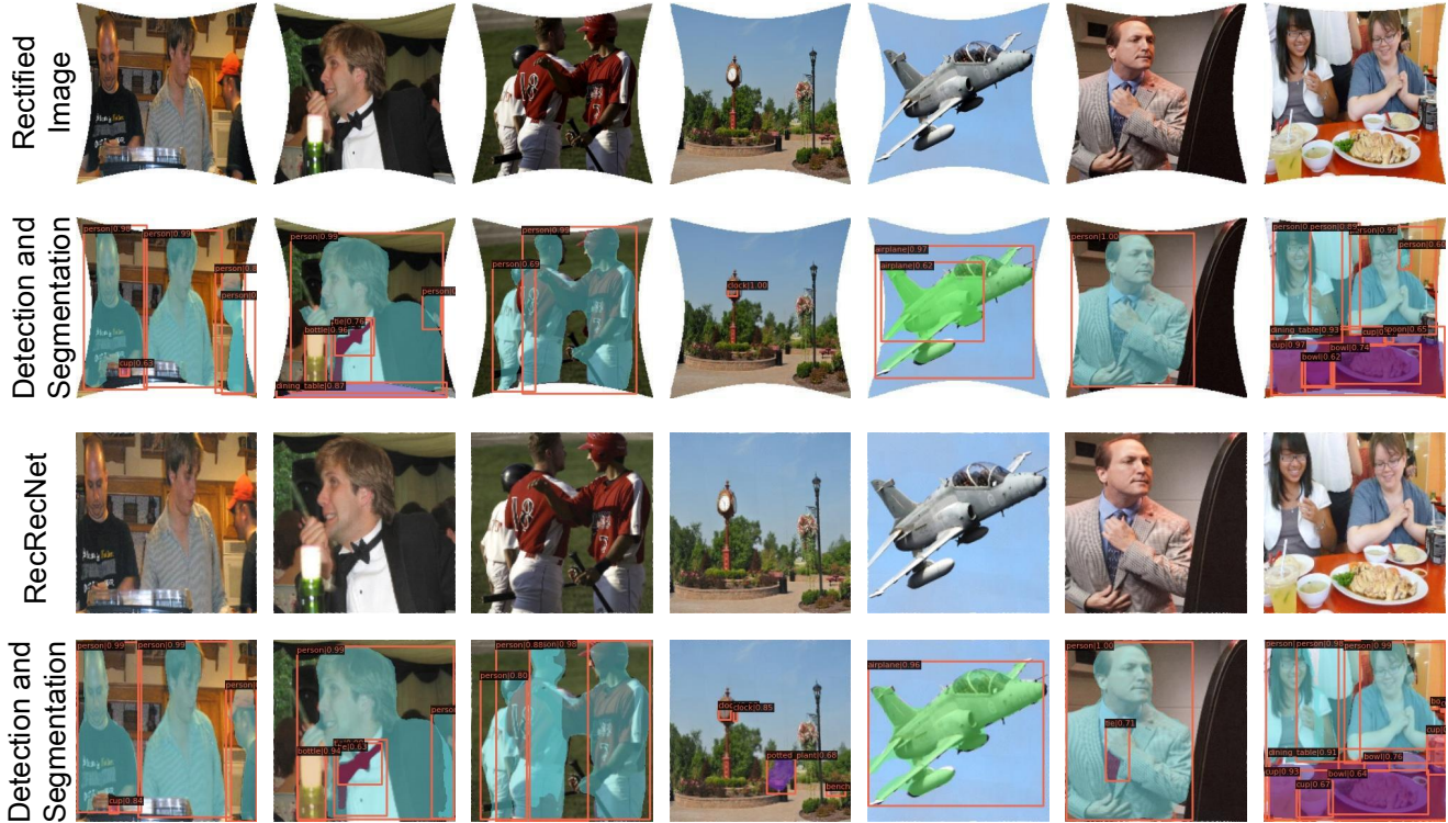
Figure 2. More detection and segmentation results by Mask R-CNN [5]. We show the rectified wide-angle image and its vision perception result, and our rectangling result and its vision perception result, from top to bottom.
